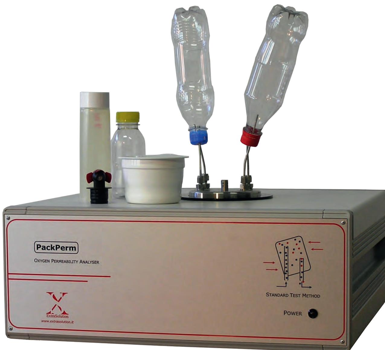
Oxygen Permeability tester. Packperm is a tester of permeability to oxygen (O<sub>2</sub>TR) for plastic bags, small containers, PET bottles, taps in bag-in-boxes, natural and synthetic crown or bottle corks and other products for packaging applications
